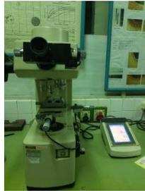
Gambar 6. Mikro hardness tester
