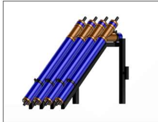
Gambar 4. Desain Mesin Multi Archimedes Screw Turbine (Parallel)
