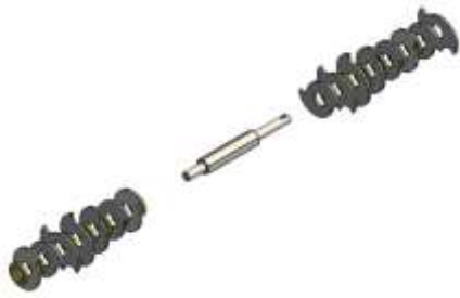
Gambar 4. Design For Assembly Pisau Dinamis
