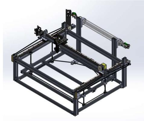
Gambar 2. Gambar Mesin CNC Laser tube Co2
