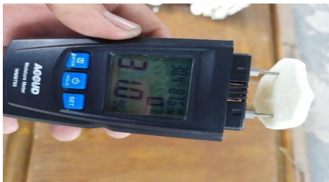
Gambar 5. Proses pengukuran kadar air awal
