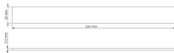
Figure 3. Dimensions of test specimens (ASTM D3039)
