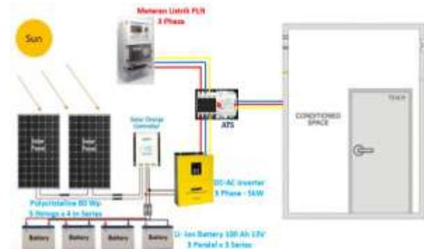
Gambar 4. Instalasi sistem solar cooling storage
