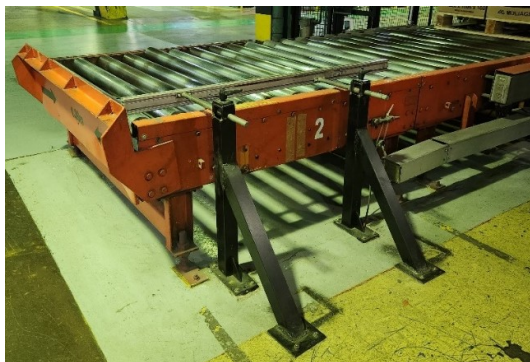
Gambar 11. Conveyor Input sesudah dipasang Stopper Pallet
