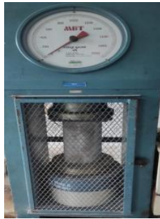
Gambar 3. Pengujian kuat tekan dimesin Compression Testing
