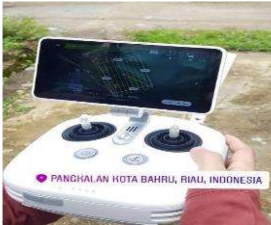
Figure 4. DJI Phantom 4 RTK Remote Controller
